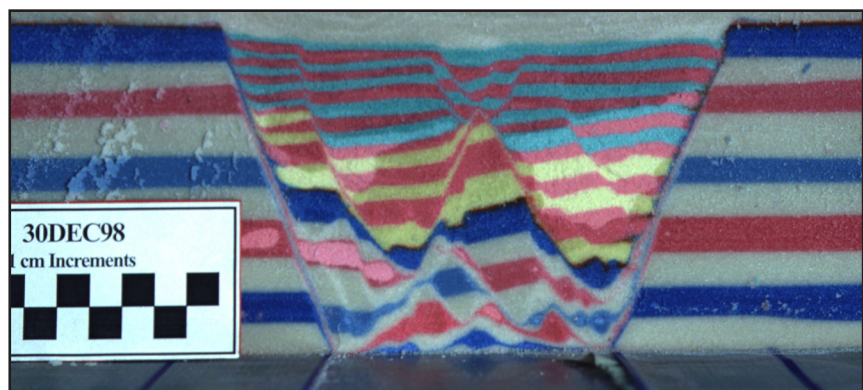
Cross-section of sand model of pull-apart basin showing graben in growth strata (blue and red) above horst earlier growth strata (yellow and red).
